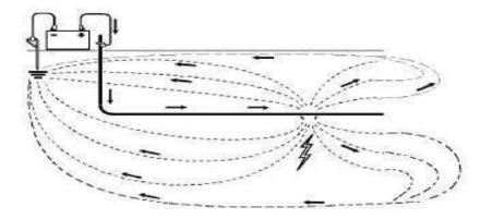
Figure 1 An A-Frame method of finding cable fault location
